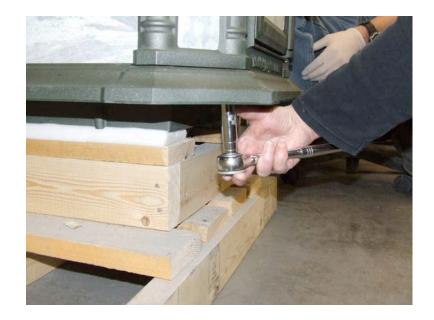
3. Locate the set screws at the center, top of the (4) cast corners on each side of the side stone and loosen them using a 1/8" hex key (Allen wrench). Remove the cast corner that holds the stone being replaced.
